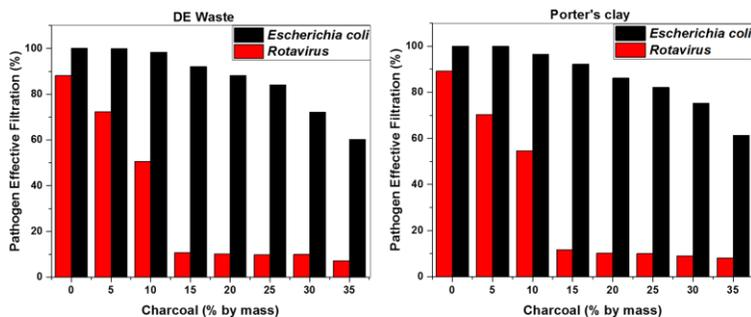
Figure 7: The percentage of pathogen filtered from water against the mass of charcoal used to fabricate the filter
