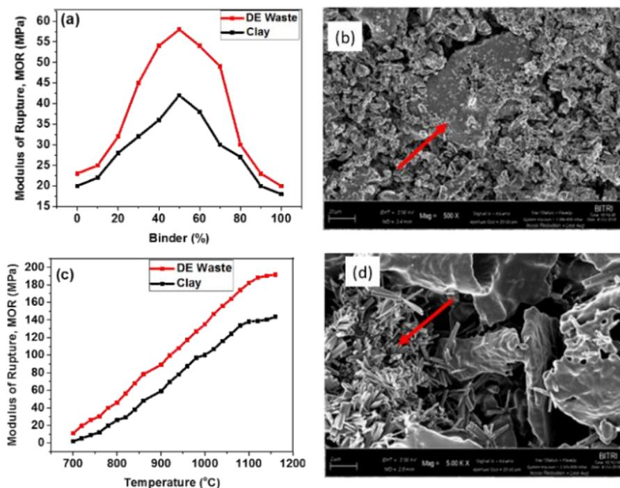
Figure 5. The plot of modulus of rupture (MOR) against binder concentration for diatomaceous earth waste fired at 900.0 °C (a) and its micrograph (b). The arrow on the micrograph show the vitrification process that took place during firing. (c) shows how the MOR varied with firing temperature and (d) shows the micrograph of the diatomaceous earth waste membrane fired at 1000.0°C. The arrows on the micrograph show the growing crystals of wollastonite
