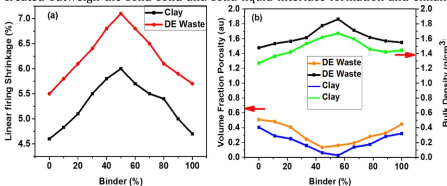
Figure 4. The effect of variation of binder on linear firing shrinkage (a), and (b) volume fraction porosity and bulk density for diatomaceous earth waste membranes fired at 900.0 °C
