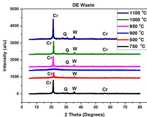
Figure 3. X-ray characteristic spectra of membranes of diatomaceous earth waste fired at (a) 750.0 °C, 800.0 °C, 950.0 °C, 900.0 °C, 1000.0 °C, and 1150.0 °C
