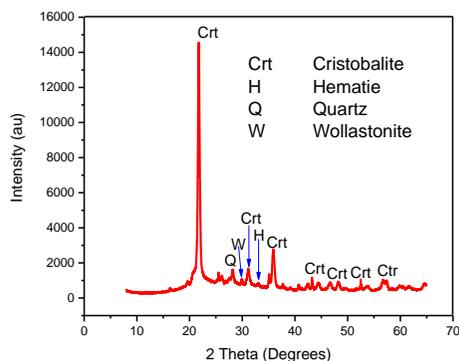
Figure 2. X-ray diffraction pattern of diatomaceous earth waste powder
